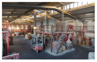
At the site in Mühlheim am Main, there are a total of six twin-screw extrusion lines for the production of through-coloured compounds for high-quality niche applications.
